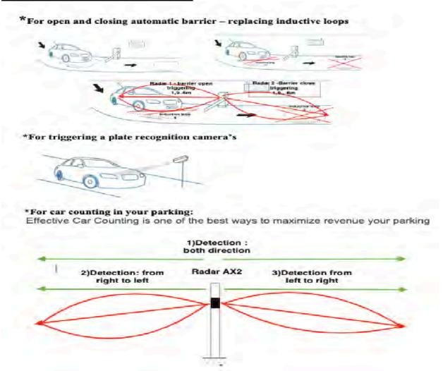
. alternative for inductive loops/photocells: contactless open-close detection Example: Speed gates in very low  $t^\circ$  - cool rooms — open and closing speed gate
